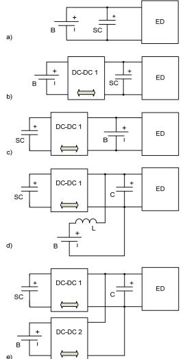
Fig. 1 The variations of the power circuit topologies of HESSs
