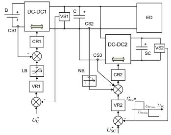
Fig. 2 The proposed control system of HESS
