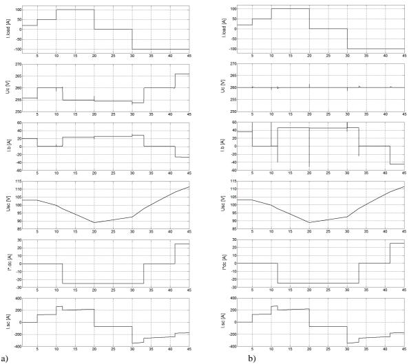
Fig. 3 The results of simulation of HESSs with the topology shown in Fig. 1d (a) and in Fig. 1e (b) as basic coordinate responses (from top to bottom):  $i_{\text{load}}$ ,  $u_{\text{C}}$ ,  $i_{\text{B}}$ ,  $u_{\text{SC}}$ ,  $I_{\text{DC2}}^*$ , and  $i_{\text{SC}}$
